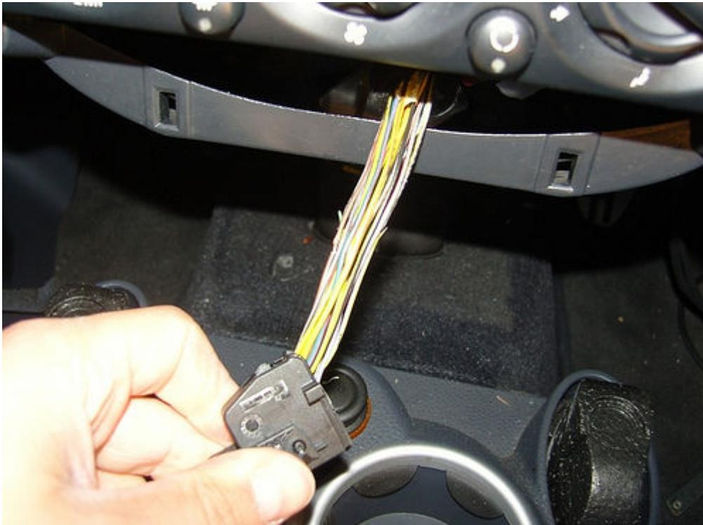
You will need to find 2 cables, the first a **brown cable with a black line** on it, and the second a **grey cable with a blue line**. Once you have found these cables you will need to cut away some of the plastic covering to expose the copper cable. Do this by carefully shaving away the plastic
