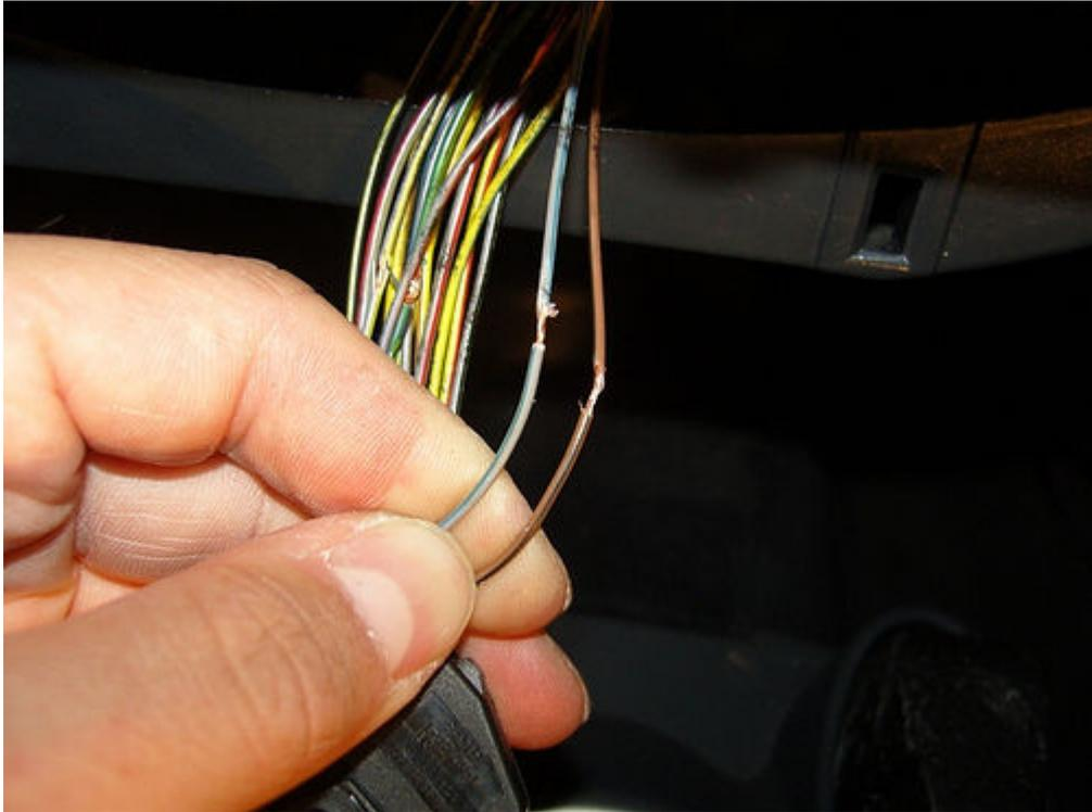
You will now need to connect the module you have made to these cables. The **black cable** from your module will need to connect to the **brown and black cable** on the car, and the **red cable** from your module will need to connect to the **grey and blue cable** on the car
