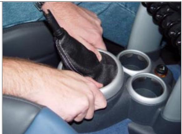
**STEP 10.** Pry the 3 tabs on the shifter cup using 2 small Flat head Screwdrivers simultaneously.
