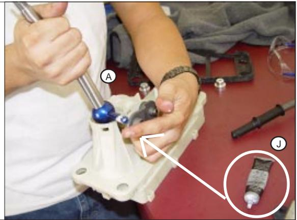
**STEP 19.** Install **B&M Pivot Cup (G)** to pivot ball of the **B&M Stick (A)** by pressing down on a hard table/surface.
