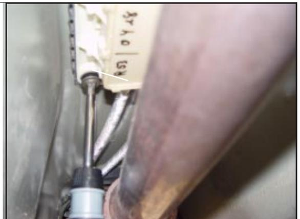
**STEP 14.** Remove stud/bushings (4) assembly from the shifter base.
