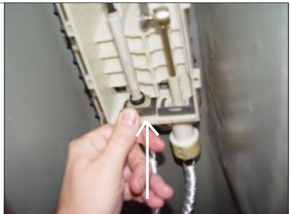
**STEP 22.** Re-install the original pivot retainer into the shifter base by aligning the 3 tabs and locking them in.
