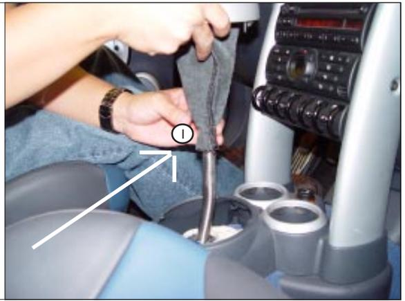
**STEP 27.** Install the stock knob by pressing down firmly (**B&M Knob** ② is optional). Press down the shift boot bezel into the shifter console.
