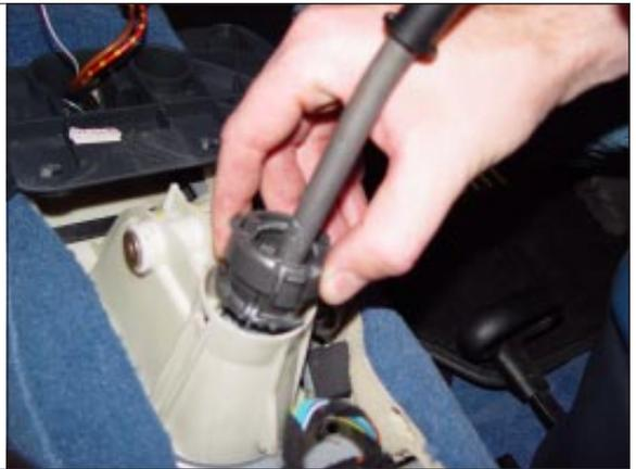
**STEP 12.** Maneuver the shifter stick and pivot arm in opposing directions. Pull up on the shifter stick to remove.
