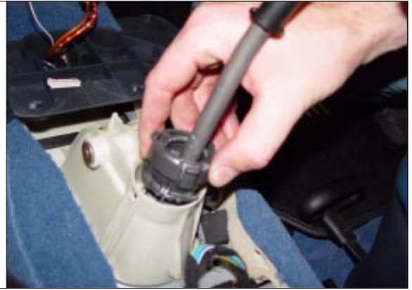
**STEP 23.** Re-install shifter cables to the pivot balls using pliers. Press the bottom shifter plate back onto the shifter base.
