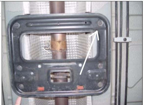
**STEP 26.** Re-attach shift boot with a tie-strap ①.
