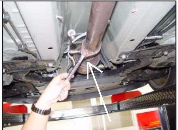
**STEP 25.** Re-attach the (2) rubber exhaust hangers and the exhaust support plate. Bolt the (6) exhaust support plate bolts. Also, re-attach the (2) rear exhaust hangers located right before the muffler.
