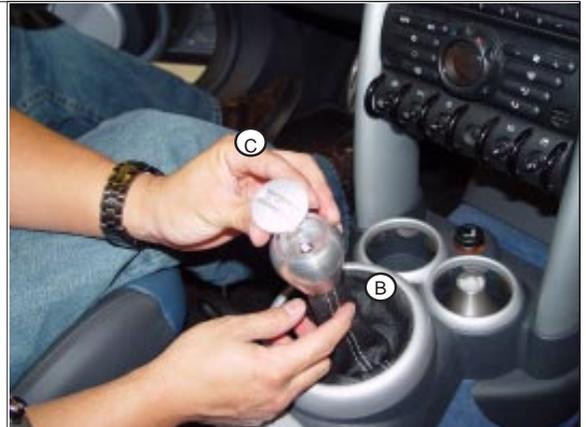
**STEP 30.** Test movement of shifter into all gears. DO NOT operate vehicle until all gears can be fully engaged smoothly.
