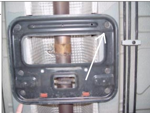
**STEP 4.** Unbolt center exhaust flange (2) bolts for easy access to the shifter. Remove the front and rear heat shields.
