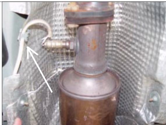
**STEP 3.** Unbolt the (6) exhaust support plate bolts. Maneuver the (2) rubber exhaust hangers and lower the exhaust support plate. Remove the (2) rubber exhaust hangers from the rear hangers near the muffler.
