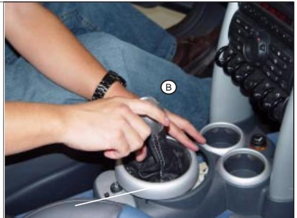
**STEP 28.** Install O-Ring (Knob) ③ onto Knob Insert ④.
