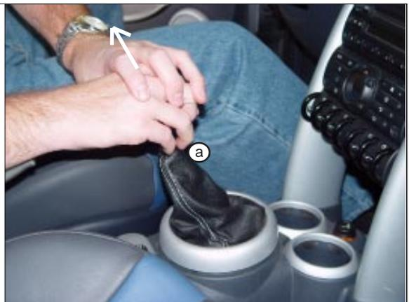
**STEP 9.** Remove shifter bezel by pulling up carefully. Cut off the tie strap to remove shift boot from the shifter stick.
